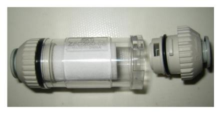
4, Clean the filter with water or compressed air
