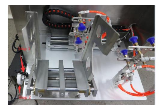
The bag magazine can be adjusted to suit for different premade bag size.
